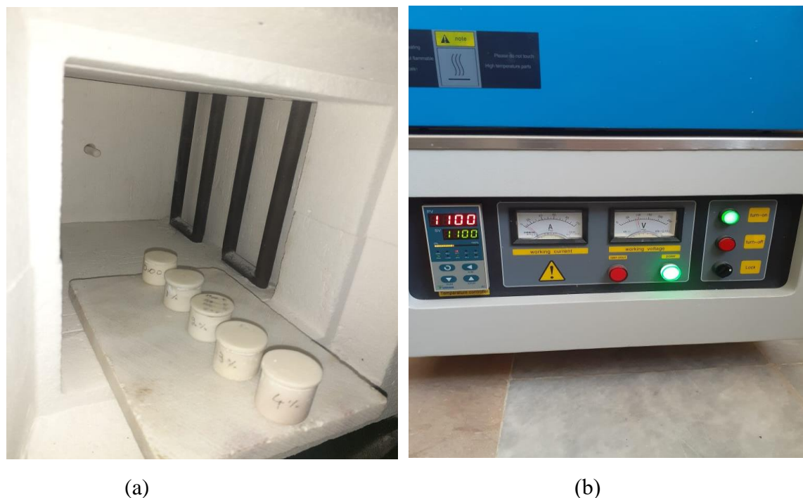
Figure 3: (a) Samples placed in furnace for calcination (b) Samples heated to 1100^{\circ}C
